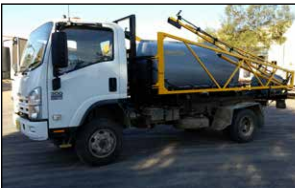
15m rear mount SmartBoom with 4 chemical tanks and 2 lockable storage cages.
