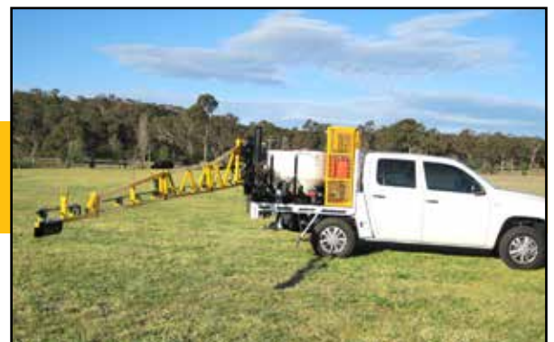
15m rear mount SmartBoom with 4 chemical tanks and 2 lockable storage cages.
