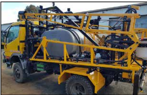
18.5m rear mount hydraulic fold SmartBoom. Custom built to suit Man truck.
