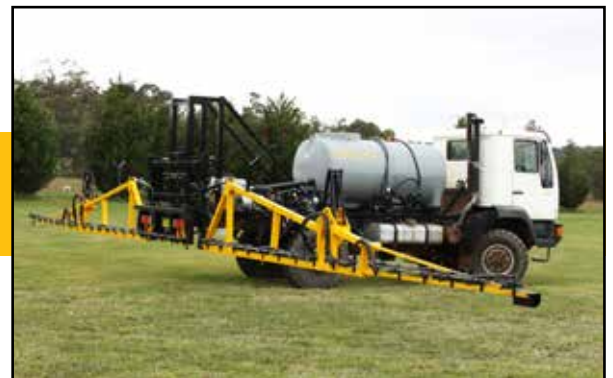
18.5m rear mount hydraulic fold SmartBoom. Custom built to suit Man truck.
